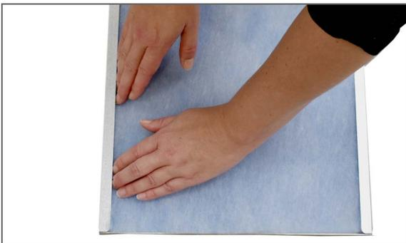
7. Press the filter sheet firmly in place in the filter frame and push it carefully towards the sides of the frame. Return the metal tracks and the filter to the unit with the filter sheet facing upwards.
