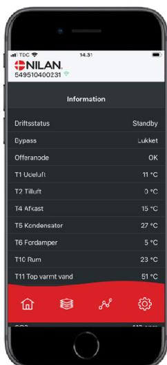
You can read off current operational data for the ventilation unit. This will allow you to check that the unit operates satisfactorily and to identify the cause of potential alarms.
