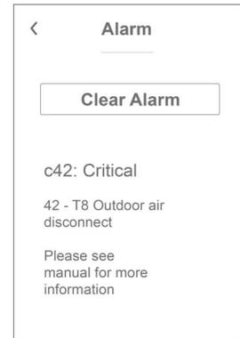
When the problem has been solved, you can reset the warning or alarm by pressing "Clear Alarm".
